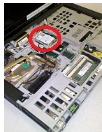
FIGURE 13. INSIDE A THINKPAD*. THE INTEL 5350 WIMAX-WIFI INTERNAL CARD IS HIGHLIGHTED
